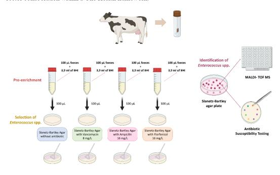
**Figure 1.** Schematic processing of cattle faecal swab samples towards the isolation, identification and characterization of *Enterococcus* spp.
